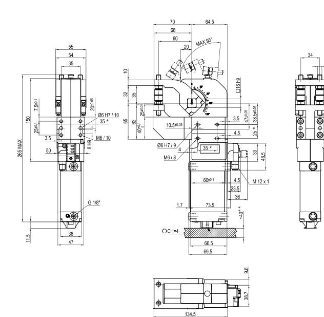
\* : TOLERANCE BETWEEN DOWELS  $\pm$  0.02, TO SCREW HOLES  $\pm$  0.1 \*\* : AREA TO ACCESS ANGLE ADJUSTMENT
