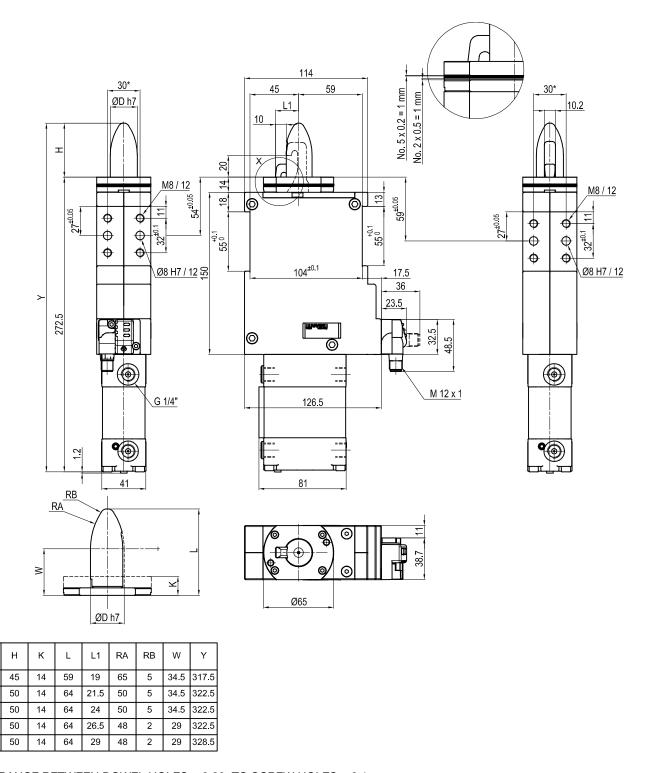
$<sup>^{\</sup>star}$ : TOLERANCE BETWEEN DOWEL HOLES  $\pm$  0.02, TO SCREW HOLES  $\pm$  0.1
